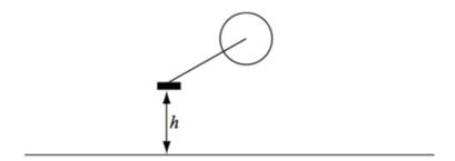
The height h cm, of the bicycle pedal above the ground after t seconds is given by  $h = 24 - 14 \sin 2t$ .
