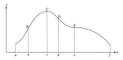
The gradient of the curve has its maximum value at point B and its minimum value at point D. The tangent is horizontal at points C and E.
