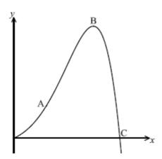
There is a point of inflexion at A, and a local maximum point at B. The curve of f intersects the x-axis at the point C.
