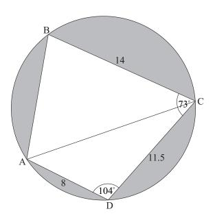
BC = 14 m, CD = 11.5 m, AD = 8 m,  $\triangle ADC = 104^{\circ}$ , and  $\triangle BCD = 73^{\circ}$
