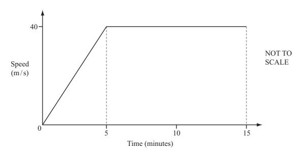
The diagram shows the speed-time graph for the first 15 **minutes** of a train journey. The train accelerates for 5 minutes and then continues at a constant speed of 40 metres/**second**.
